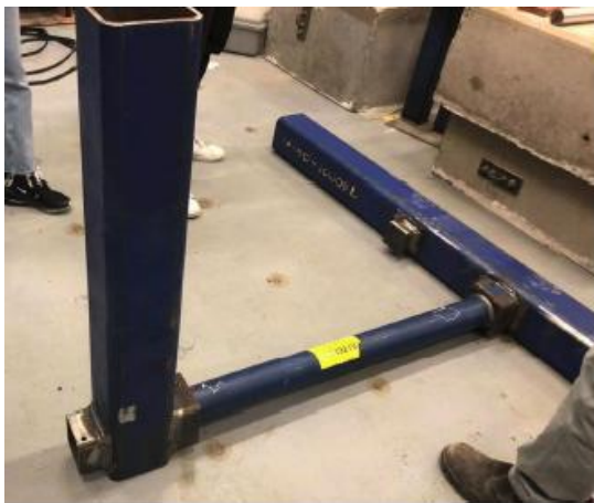
Figure 2: Torsion test assembly
