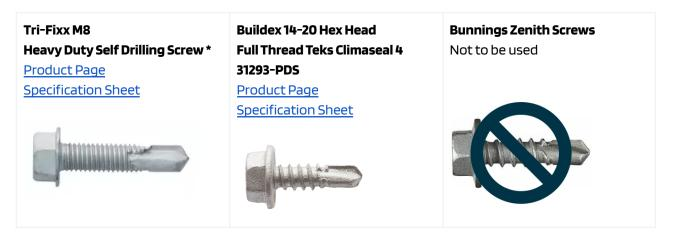
\* The Tri-Fixx M8 heavy duty screw needs to be drilled at a slower speed of less than 100rpm in order for the screw to start cutting the steel – high speed drilling of this screw will only heat treat the steel making it impossible for the screw to penetrate the steel.
