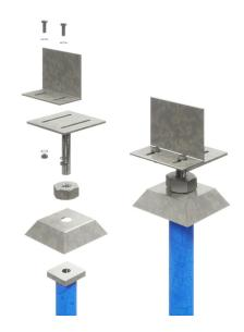
The bearer plate connector (backing plate) may clash with the chassis in the corner and joists in certain locations.
