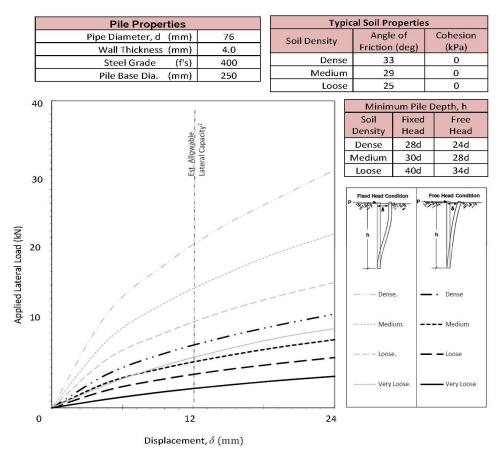
These charts are for Katana Piles only as lateral performance is highly dependent on the connections rigidity and shaft properties. It is Katana's opinion that these graphs represent a reasonable approximation of the average performance of the Katana Pile in the indexed soils. Using the average performance is reasonable for multiple redundant structures (e.g. buildings, bridges, marina piers, etc.)
