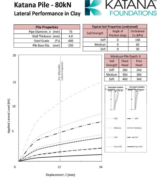
These charts are for Katana Piles only as lateral performance is highly dependent on the connections rigidity and shaft properties. It is Katana's opinion that these graphs represent a reasonable approximation of the average performance of the Katana Pile in the indexed soils. Using the average performance is reasonable for multiple redundant structures (e.g. buildings, bridges, marina piers, etc.)
