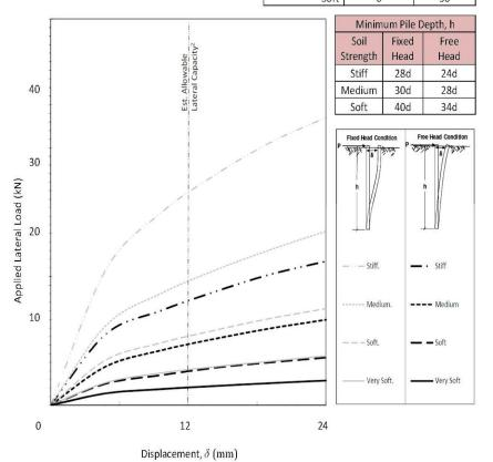
These charts are for Katana Piles only as lateral performance is highly dependent on the connections rigidity and shaft properties. It is Katana's opinion that these graphs represent a reasonable approximation of the average performance of the Katana Pile in the indexed soils. Using the average performance is reasonable for multiple redundant structures (e.g. buildings, bridges, marina piers, etc.)
