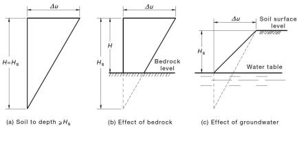
$\Delta u$  and  $H_{\rm s}$  are to be taken from Table 2.4 (except that  $H_{\rm s}$  is taken as the depth to water table if it is less than the value in Table 2.4)
