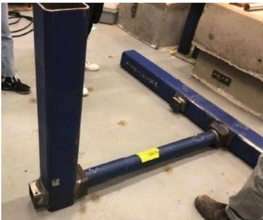
**Figure 2: Torsion test assembly**
