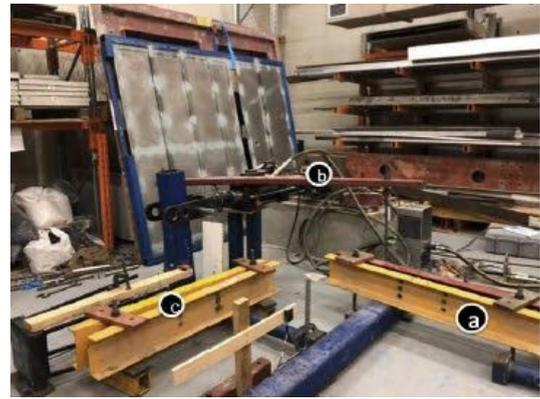
**Figure 3: Restraints applied to the testing system**
