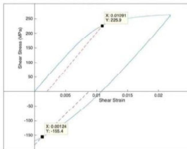
**Figure 4: Prediction of elastic yield by using a 0.2% offset**
